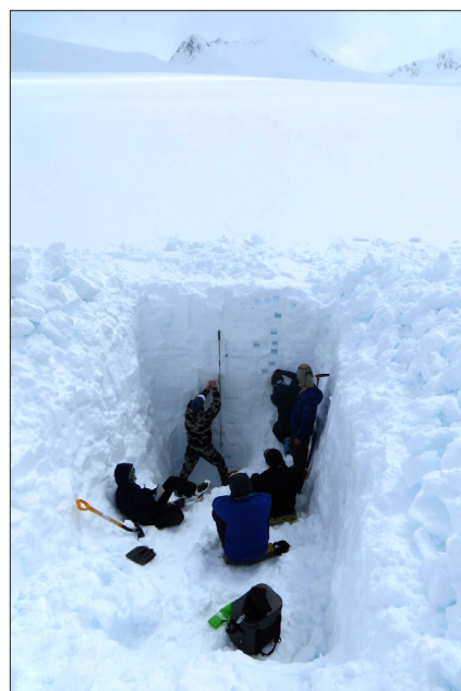
Students atop Eklutna Glacier dig a pit to measure snow density. Photo by Jason Geck.
